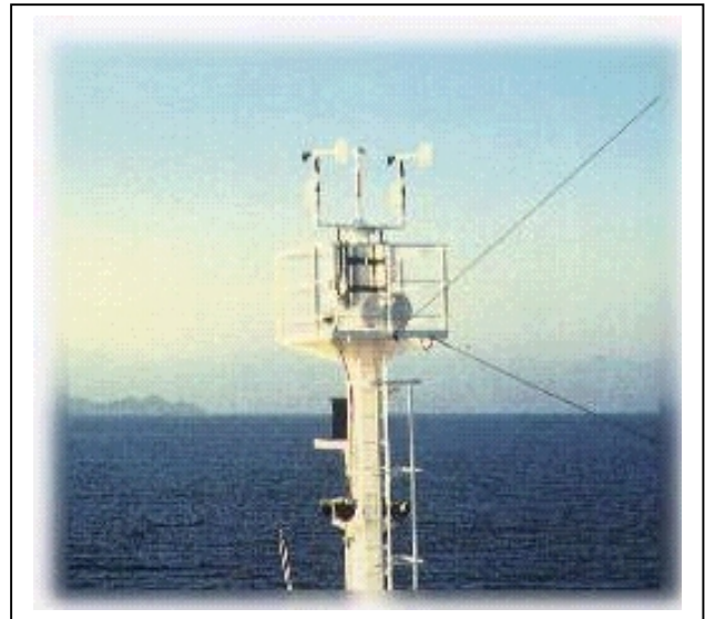
FIGURE 1: Photo of the sensors and intelligent interface assemblies on the foremast of the R/V ALLIANCE . The fiber optic and power cables are protected in flexible coated metal conduit. Photo courtesy of Dr. Peter Minnett
