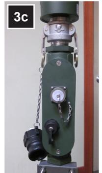
4. Place the entire unit (upper tower section and WEATHERPAK™) onto the tripod and turn clockwise to secure. Hand tighten the screw.
