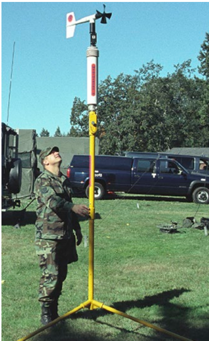
WEATHERPAK® on portable three meter tower
