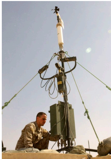
Military WEATHERPAK® with additional visibility sensor
