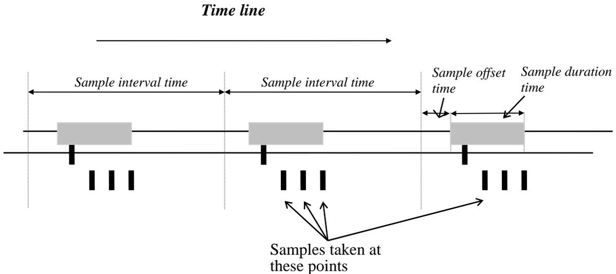
The sample interval always starts, as far as possible, at an even time -- for example, if the sample interval time is one hour then the sample intervals start on the hour. The sensor outputs are sampled throughout the sample duration time.
