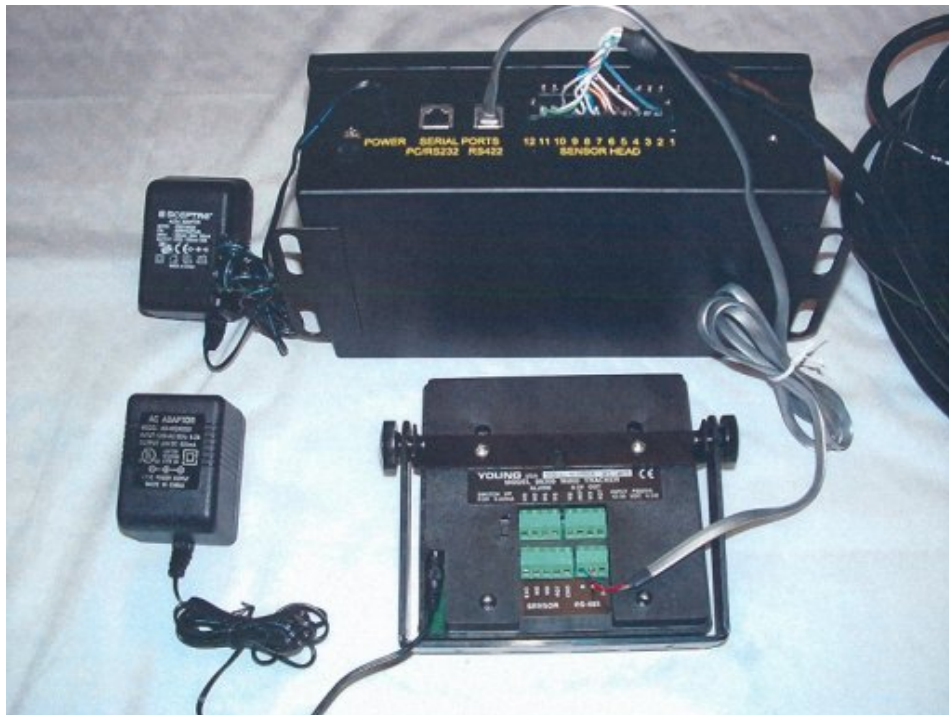
C-5 SAM/N showing all interconnections: top: side view of C-5 SAM/N display box (shown in top photo at bottom left), top-left: C-5 SAM/N power supply, bottom and bottom-left: optional Repeater and Repeater power supply.
