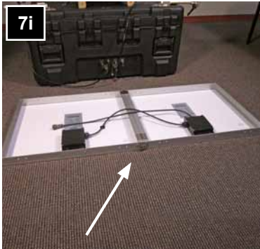
Open up the solar panels as shown above. Lock the two panels by turning the attached screw.
