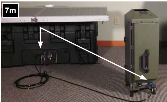
Place the ceilometer on level ground near the main case; attach the cord to the bottom right connector on the sensor, and to the connector on the top left of the main case.
