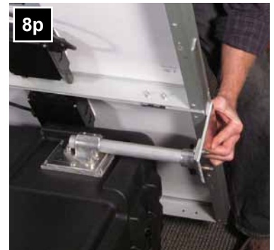
Push the solar panels until the pins are inserted into the holes as far as they go.
